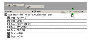
Figure 3.3: Removing grouped items: Removing the Type group
